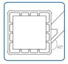
For angled rail installations - align angled face of Support Block parallel to rail section.
